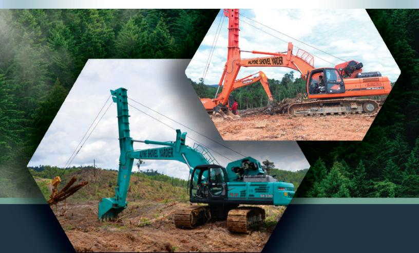
DOUBLE DRUM HYDRAULIC INTERLOCK IS CAPABLE OF OPERATION WITHOUT THE NEED OF GUY LINES. THESE VERSATILE YARDERS CAN YARD UPHILL AND DOWNHILL. THIS HIGHLY MOBILE YARDING SYSTEM MEETS TODAY'S DEMANDING LOGGING REQUIREMENTS.
