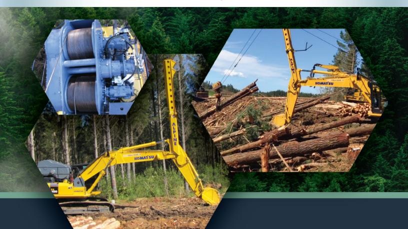
DOUBLE & TRIPLE DRUM SYSTEMS ARE CAPABLE OF OPERATION WITHOUT THE NEED OF GUY LINES. THESE VERSATILE YARDERS CAN YARD UPHILL AND DOWNHILL. THIS HIGHLY MOBILE YARDING SYSTEM MEETS TODAY'S DEMANDING LOGGING REQUIREMENTS.
